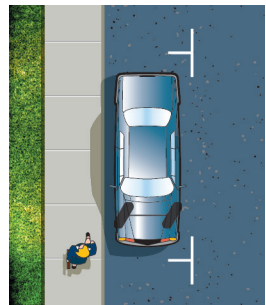
Downhill with curb: Steering wheel turned right.
