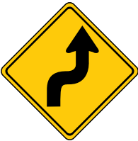
Reverse curve ahead Two turns in opposite directions separated by a tangent of less than 120m, first turn right
