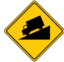
Steep hill ahead Shift to lower gear or slow down if going down very steep hill
