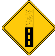
Pavement ends Continuation has gravel surface
