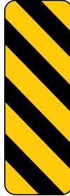
Hazard close to the edge of the road The downward lines show the side on which you may safely pass
