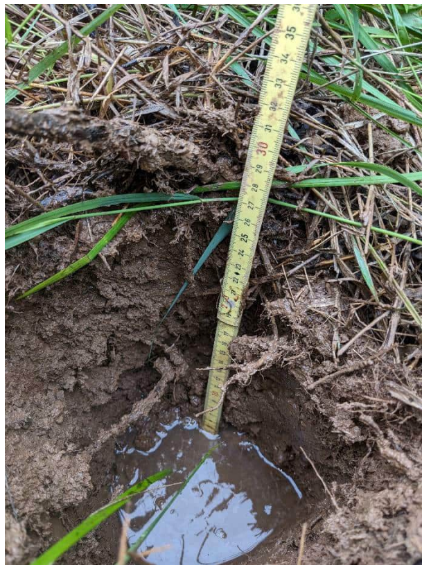
WL2 Photo 4 – Displaying Depleted Matrix (5YR 4/2 90%, 5YR 5/6 10%) at 0-30 cm for WL2
