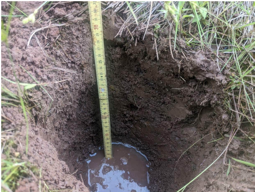
WL1 Photo 4 – Displaying Depleted Matrix (5YR 4/2 80%, 5YR 4/6 20%) at 0 – 30 cm for WL1
