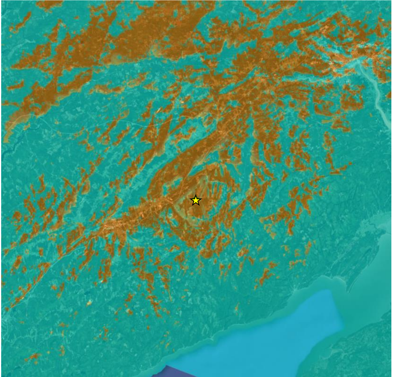
Figure 5-5: Zone of Visual Influence over a 48km visual analysis radius. Yellow color demonstrates some portion of the turbine may be visible.
