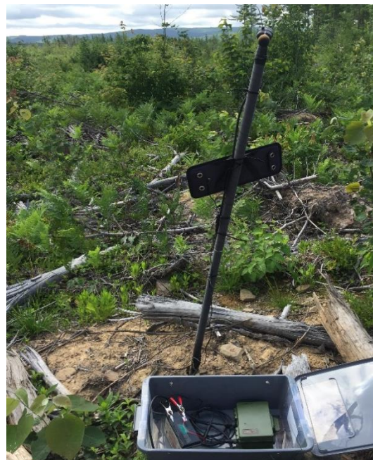
Figure 3-5: Acoustic Bat Detector Setup
