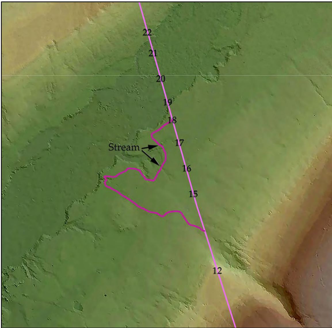
Figure 4: Approximate locations of transmission line structures and access road on LiDAR image.
