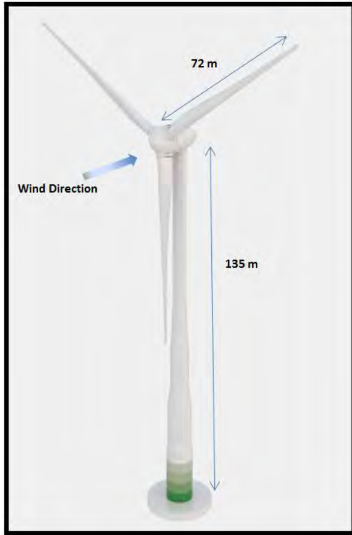
Figure 3: Anticipated Turbine Hub and Blade Lengths
