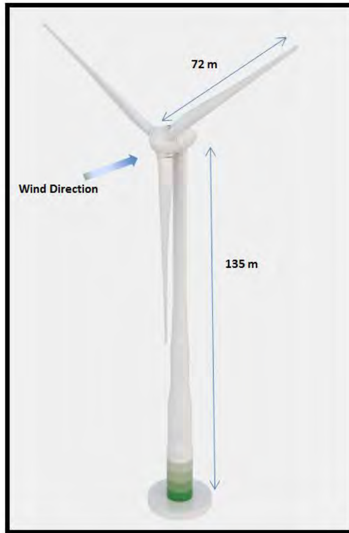
Figure 3: Anticipated Turbine Hub and Blade Lengths
