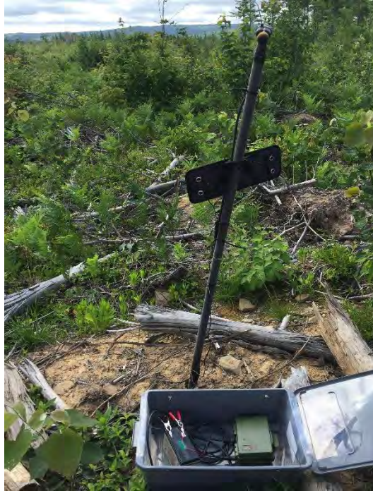
Photo 2. Wildlife Acoustics SM4BAT ultrasonic bat detector and condenser microphone used at station 1.
