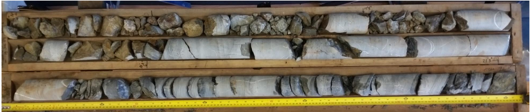
Photograph 1 – Rock Core BH-1 – 1.75 ft to 12.25 ft below mudline
