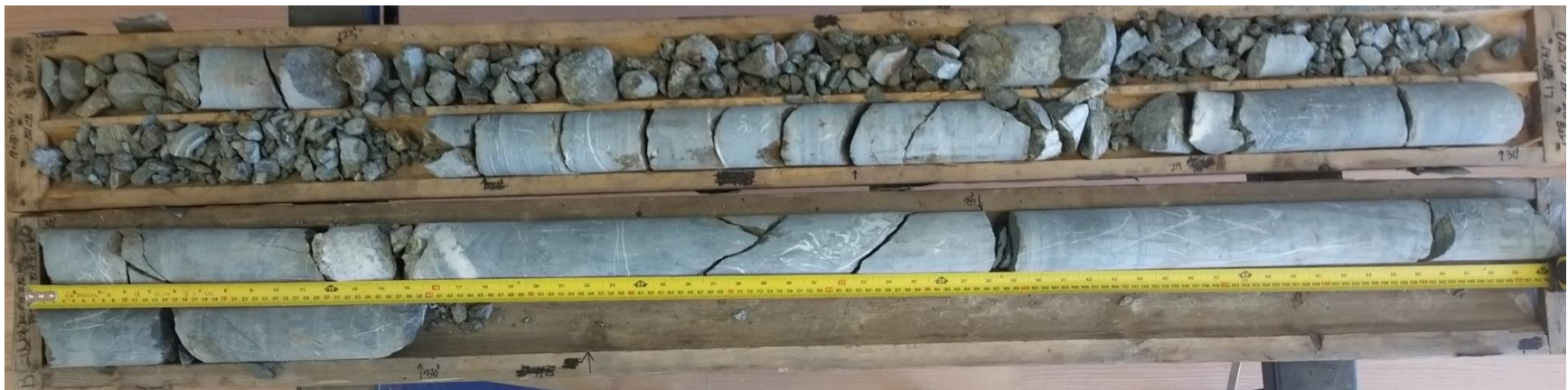
Photograph 2 – Rock Core BH-2B - 22 ft to 36 ft below mudline
