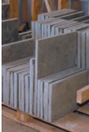
Stone is a very adaptable medium. It can be utilized in its natural state or cut into building blocks for office towers, manufactured into curbing stone or carved into ornate sculptures. These and countless other items are made of what we call dimension stone, or rock which has been shaped and/or finished.
