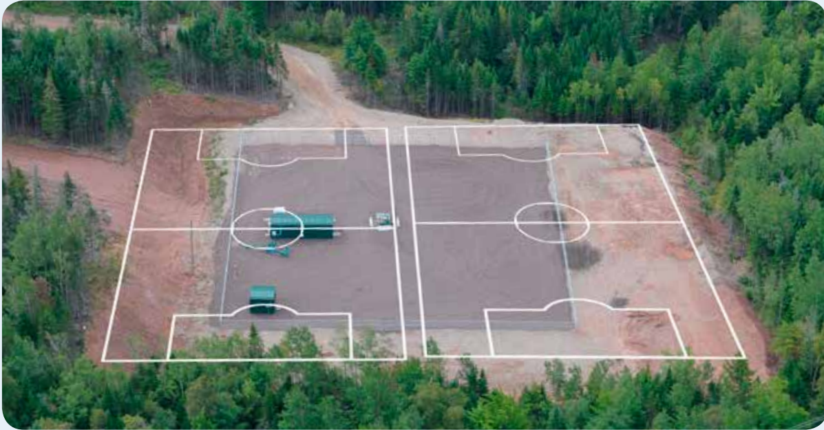
A Corridor Resources well pad in New Brunswick during the production phase. Outlines of soccer fields shown for size comparison.
