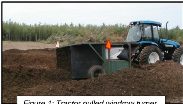
Figure 1: Tractor pulled windrow turner
