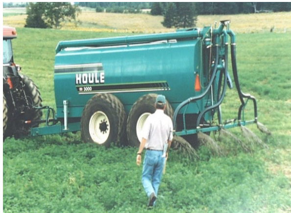
Figure 1. Rear mounted boom spreader
