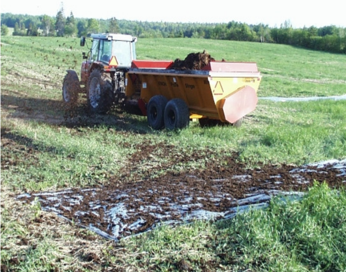
Figure 4. Side discharge manure spreader
