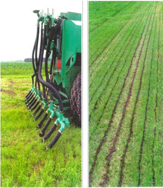
Figure 2. Drop tube distribution system and resulting manure application to soil surface
