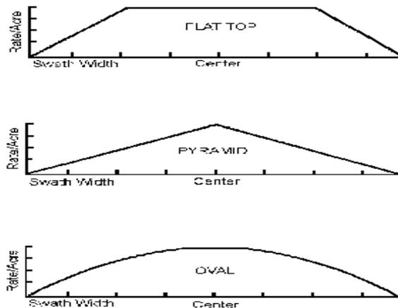
Figure 1. Broadcast spreader patterns
