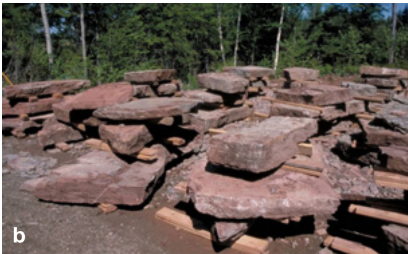
Figure 16. The laminated even bedded nature and durability of Macumber Formation limestone make it a very suitable natural material for a wide range of construction stone products. Photo a shows pallets of processed flagstone and wall-stone typically used in landscaping and various building application. Photo b shows stone typically used for stepping stones, stair treads, and armour stones.
