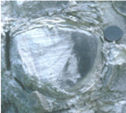
Figure 27. The formation of spherical sulphate (anhydrite/gypsum) structures, referred to as cannonballs, results from the subsurface chemical weathering (hydration) of anhydrite. Concentric shells of hydrated gypsiferous rock are successively loosened and separated from a block of anhydrite as water penetrates bounding joints or fracture systems and attacks the block from all sides. These structures indicate proximity to significant water bearing fault zones and mark the outer limit of hydration fronts in the Wilson Brook-Demoiselle Creek area, Albert County, southeastern New Brunswick (after Webb 2002a, b).
