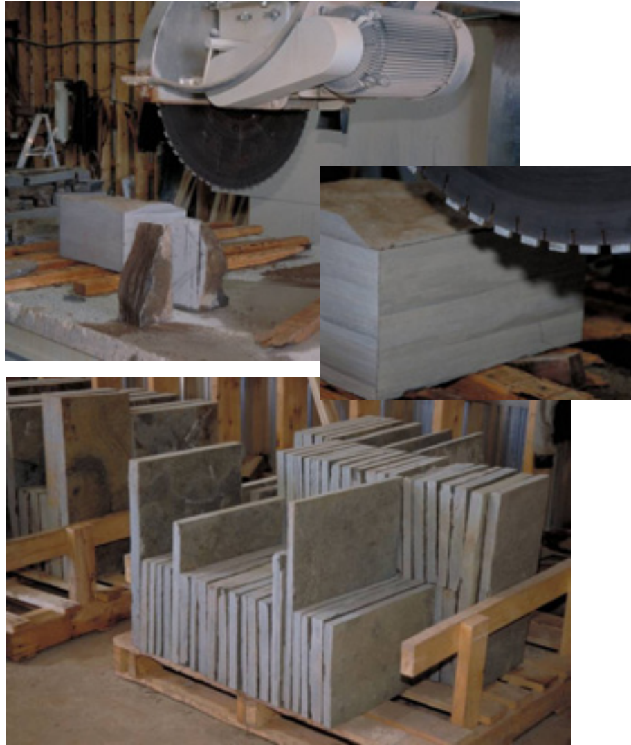
Figure 17. Using a selection of custom stone cutting and shaping equipment, including a computerized diamond rotary saw and hydraulic stone splitters, Brunswick Limestone Ltd. produces several cut and guillotined stone products in addition to variously sized, randomly shaped products.
