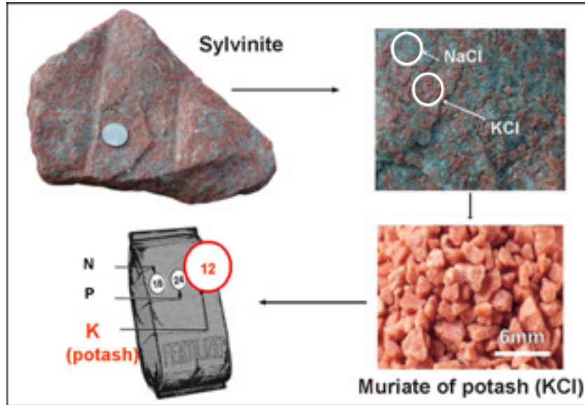
Figure 45. In New Brunswick, potash ore (sylvinite) is primarily a mix of potassium chloride (sylvite, KCl) and sodium chloride (halite, NaCl). The commercial products produced from sylvinite ore are referred to as muriate of potash or KCl. Virtually all potash production finds its way into the agricultural sector in the form of a major fertilizer ingredient symbolized as the “K” ingredient on most commercial bags and containers.
