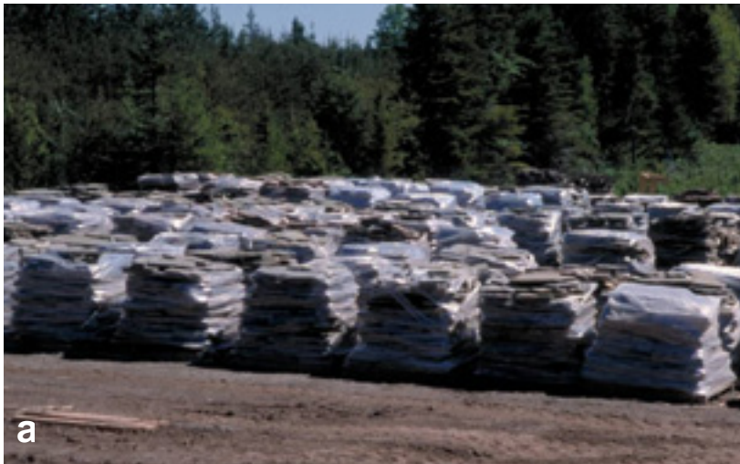
Figure 16. The laminated even bedded nature and durability of Macumber Formation limestone make it a very suitable natural material for a wide range of construction stone products. Photo a shows pallets of processed flagstone and wall-stone typically used in landscaping and various building application. Photo b shows stone typically used for stepping stones, stair treads, and armour stones.
