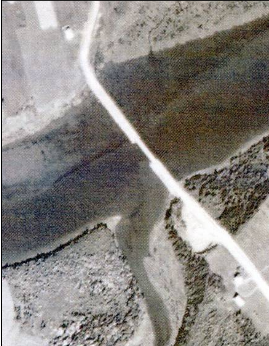
Figure 12. 1955 Aerial of Little Tracadie River bridge built in 1949. Note the new position of the river channel. (NBDNR 1955-3900-286) North at top of photo.
