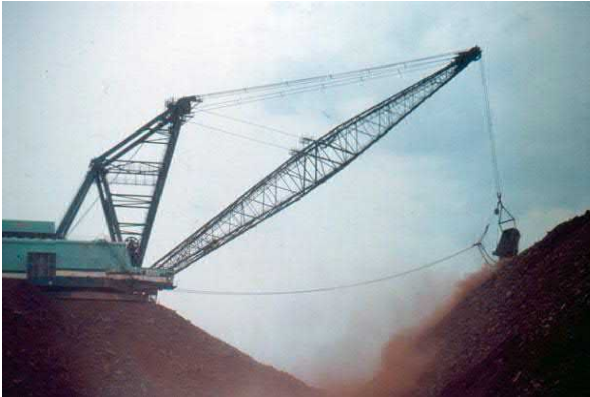
Photo no. 1. NB Coal cable dredge operating (NB Museum, 2012).
