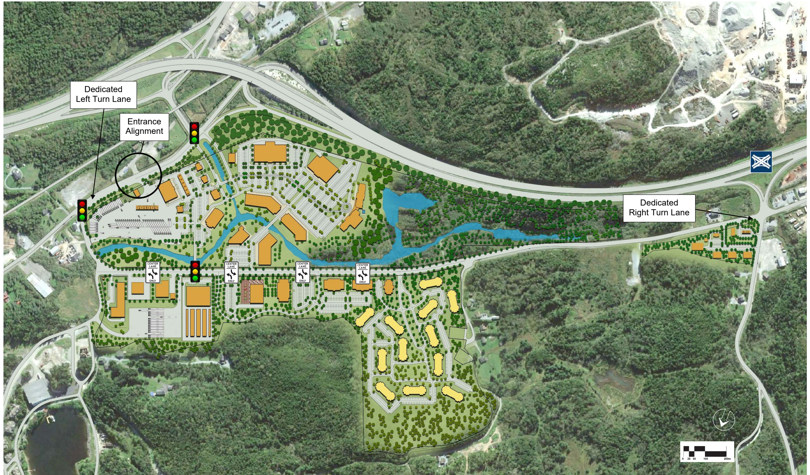
Figure 10. Improvements and upgrades recommended by exp Services Inc. [2017a] to the existing road network to improve traffic flow in the vicinity of The Crossing in east Saint John, New Brunswick.
