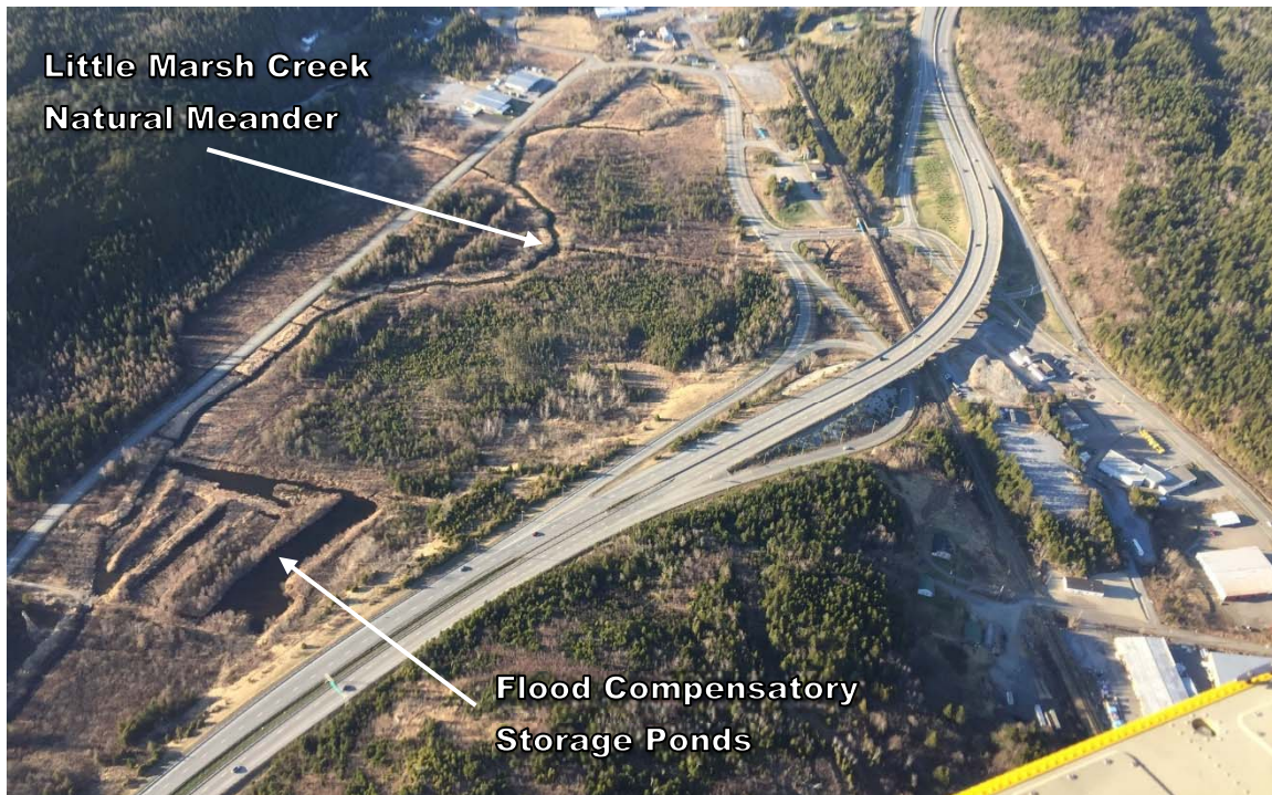
Figure 5. Aerial photograph showing two key environmental features at The Crossing site in east Saint John, New Brunswick.
