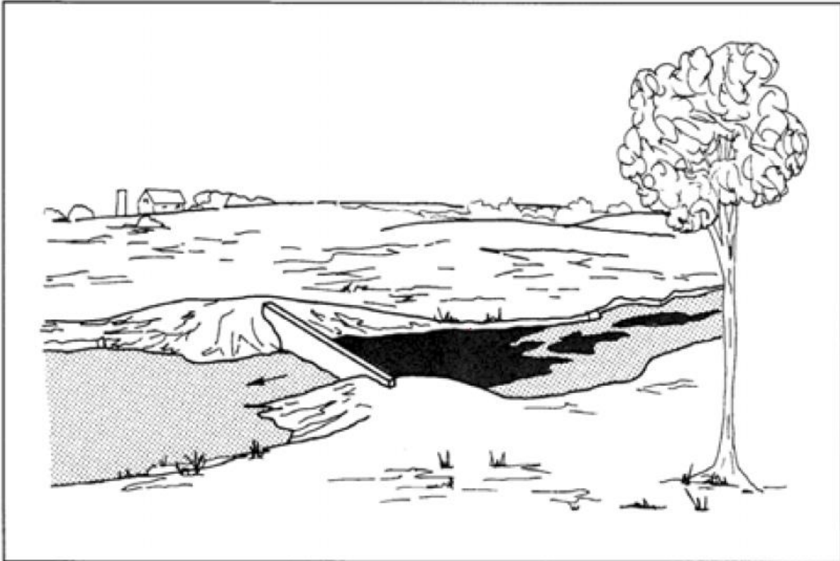
Use of culvert weir on a small watercourse.
