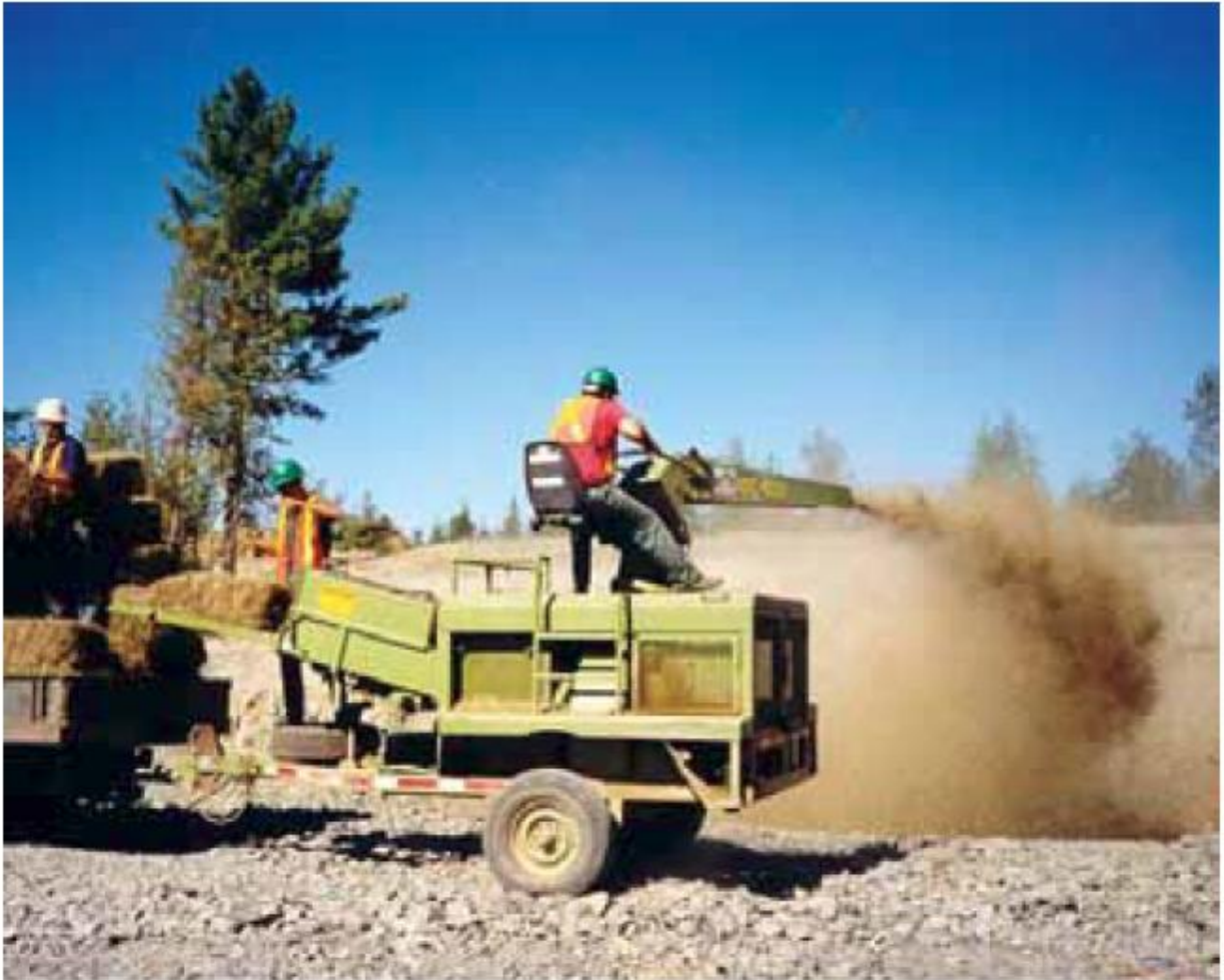
Mulching – Application by mechanical means.
