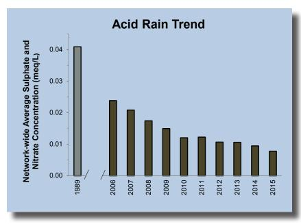
The key indicators for acid rain are sulphate and nitrate concentration. Each of these parameters has a slightly different effect on acidity, but can be combined and expressed as "milliequivalents per litre" (meq/L). As reflected in the chart to the left, peak levels occurred in 1989. Emission reduction strategies have reduced sulphate and nitrate concentrations by approximately 81% since then, and the trend is continuing.
