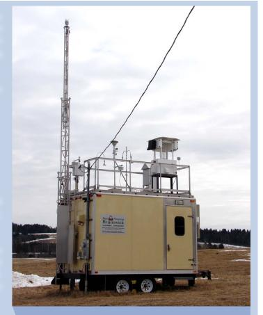
The DELG mobile air quality monitoring unit (pictured above) is typically equipped with monitors for:
